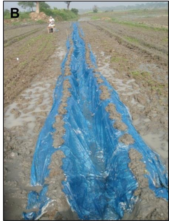
Supplemental Figure S1. Field Pictures. A. 45-cm-wide, 45-m-long control channel prior to experimentation. B. Tarp-lined, soil-free channel, prior to experimentation. Plastic tarp was held down with mounded soil on the top of channel walls. C. 1x-, 2x-, and 3x-width channels, prior to experimentation. D. Turbid irrigation water flowing along the wetting front in a 3x-width channel.
